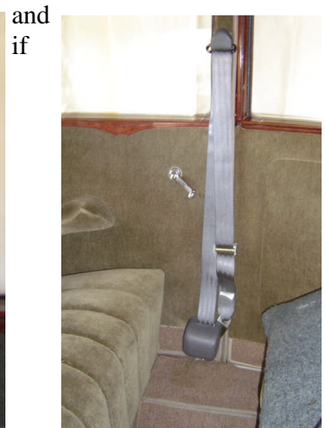
Figure 5 Driver's Seat Belt showing retractor installation
